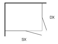
Corner shower enclosure composed of two sides, each consisting of a fixed door hinged to a swing door provided with aluminium glazing bead bars
