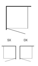
Corner shower enclosure with wall-mounted hinge, consisting of a hinged door and a fixed side panel with glazing bead bar
