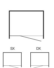
Niche door composed of a fixed door hinged to a swing door provided with glazing bead bars.
