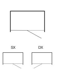
Niche door composed of a fixed door hinged to a swing door provided with a glazing bead bar
